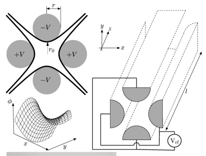
A schematic of an ideal hyperbolic electrostatic quadrupole (thick line) circular the and electrodes used to closely approximate the hyperbolic shape are shown on the top left. The saddle-shaped harmonic potential it creates is illustrated at the bottom left. The geometry formed from half-cylindrical rods and pair-wise applied a.c. potential (Vrf).
