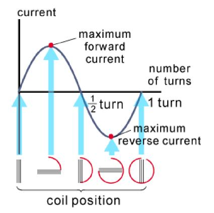
Notice that the voltage WILL alternate or have ripples even if the contacts to the terminals are flipped every half cycle Inductors and generators : The simple generator : coil rotates, magnet stationary
